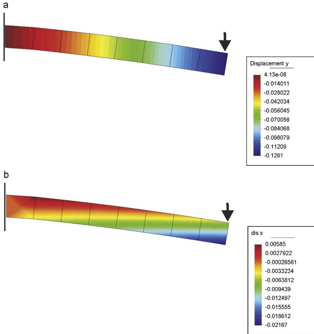
Fig. 6. Cantilever beam subjected to a tip load of 200 kN: results at the master node corresponding to the external loading position: (a) vertical displacement (m); (b) horizontal displacement (m).
