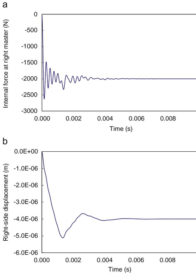
Fig. 3. Compression test: results at the master node corresponding to the external loading position: (a) internal force; (b) displacement.
