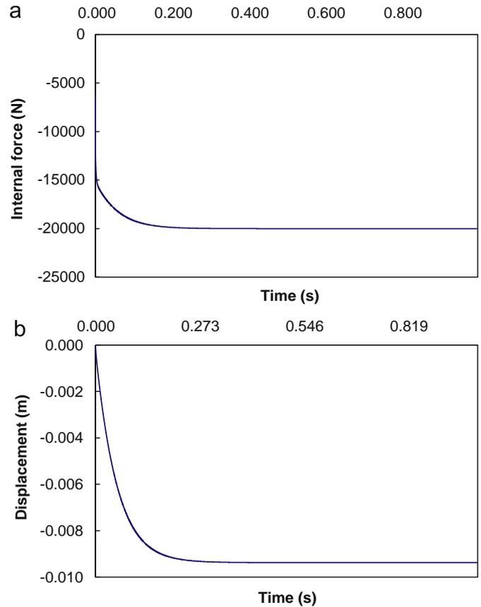
Fig. 4. Cantilever beam subjected to a tip load of 20 kN. Results at the master node corresponding to the external loading position: (a) internal force; (b) vertical displacement.
