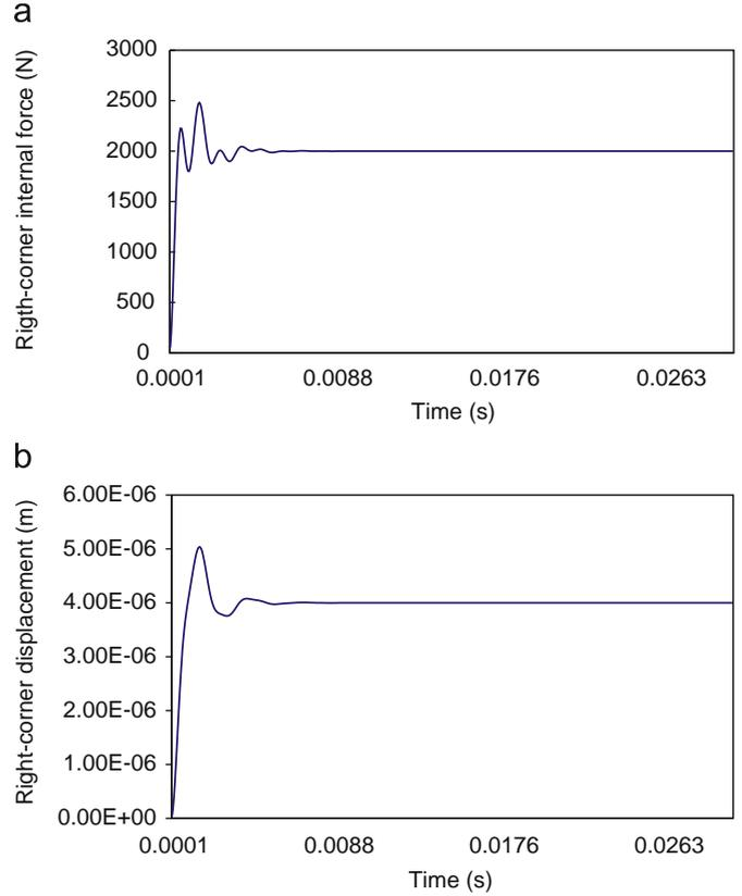
Fig. 2. Tension test: results at the master node corresponding to the external loading position: (a) internal force; (b) displacement.
