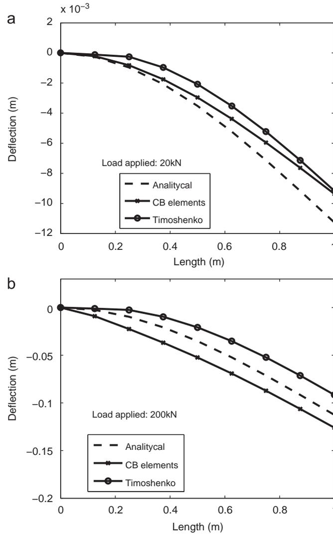
Fig. 7. Deflection along the cantilever for two different load tips. Comparisons are made against simulation by Timoshenko beam elements and analytical solution: (a) 20 kN; (b) 200 kN.
