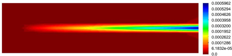
Fig. 9. Continuum—modelled as a softening material—from where the bar formed by CB is pulled out.
