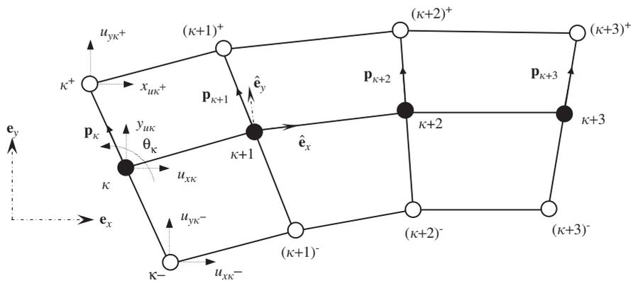
Fig. 1. The figure shows a typical continuum-based (CB) element. In this sample, it is composed of four master nodes—in bold—and eight slave nodes but other configurations are also possible.
