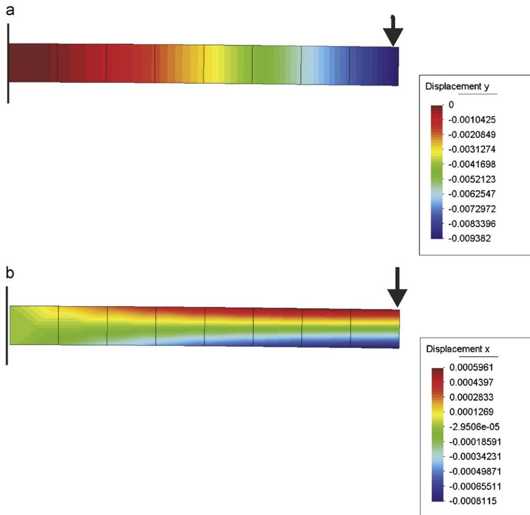
Fig. 5. Cantilever beam subjected to a tip load of 20 kN. Results at the master node corresponding to the external loading position: (a) vertical displacement (m); (b) horizontal displacement (m).
