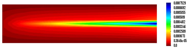
Figure 2: Displacement field contours (m) -only half of the sample is depicted- in the concrete. Displacements of the rebar nodes are not represented.
