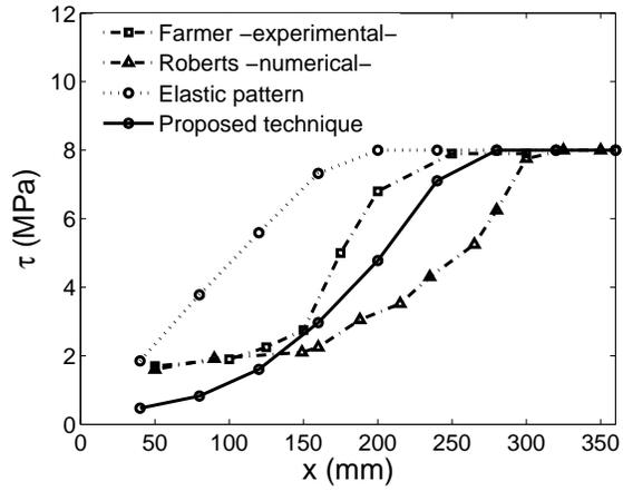
Figure 3: Numerical versus experimental bond stress along the reinforcement. External force = 100 *KN*. Elastic pattern refers to an elastic interface law assumption and it is provided for comparison purposes with the more realistic proposed law.
