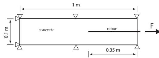
Figure 1: Details of the idealised configuration of the pullout test in a two-dimensional context
